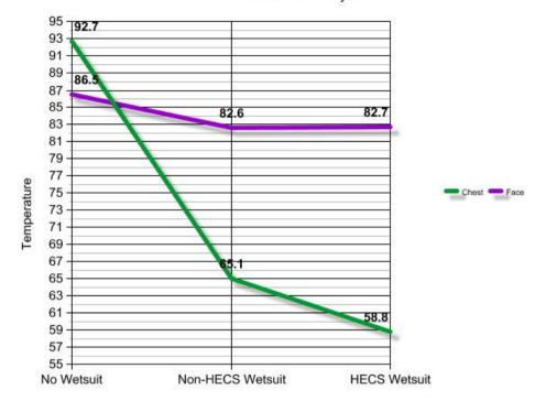
When compared with our control what we discovered here is that after 10 minutes we measured a **6.3°F** difference in the chest and a **0.1°F** difference in the face.
